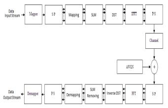
Fig. 1. The Proposed hybrid IOFDMA Model
