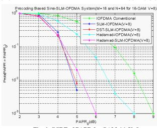
Fig. 4. CCDF of PAPR for QAM-16, V=8
